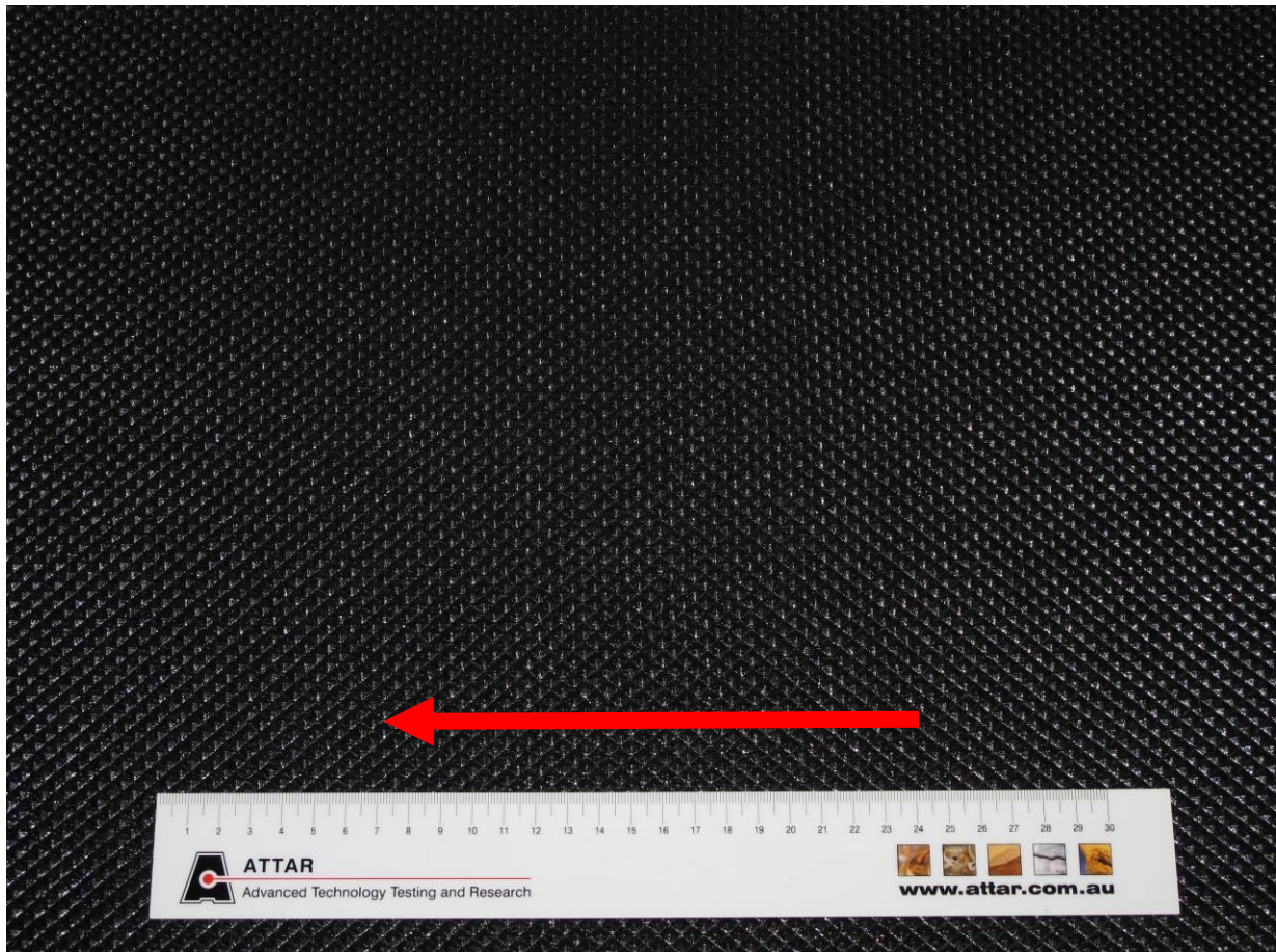
Figure 1: Stair nosing insert – PVC type ridged pyramid finish. Arrow indicates direction of test.
