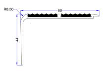
In this example, AA208 has been installed with 2mm vinyl sitting under the rebated edge of the profile. This installation has used slip resistant Tredsafe Diamondtred insert for safety, which meets standards of AS/NZS 3661.1:1991 and NZS 4586:2013.
