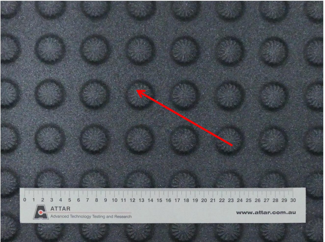
Figure 1: ALLTAC SIRUS TGSi Allgrip Finish. Arrow indicates direction of testing.
